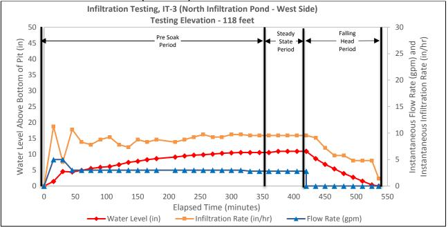
The constant-head (steady-state period) measured infiltration rates in the north infiltration pond were 7.1 inches/hour (IT-2) and 9.2 inches/hour (IT-3), for an average rate of 8.1 inches/hour. Using an intermediate correction factor for site variability, due to silt lenses, the design infiltration rate for the north infiltration pond was 0.8 inch per hour, after applying correction factors shown in Table 3.
