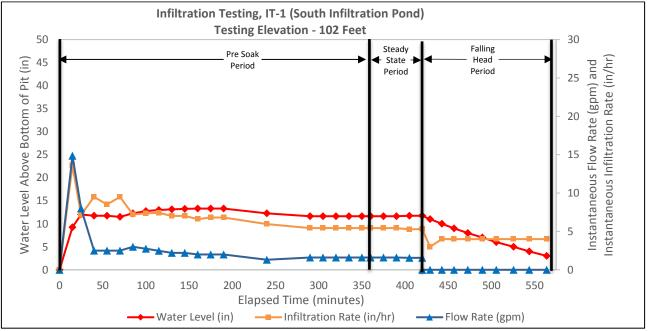
Using the constant-head (steady-state period) measured infiltration rate (1.3 inches per hour) and an intermediate correction factor for site variability, due to silt lenses, the design infiltration rate for the central infiltration pond was found to be 0.16 inch per hour, after applying correction factors shown in Table 3.
